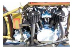
In 1930, the 74-cubic-inch (1,210 cc) VL flathead replaced the JD Big Twin, which had
